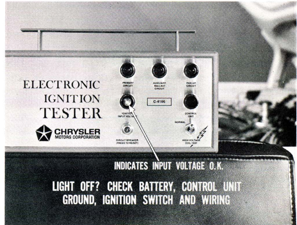
Fig. 18—Tester needs sufficient voltage to operate
