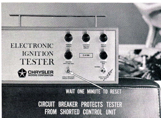
Fig. 24—Push red button in to reset circuit breaker
