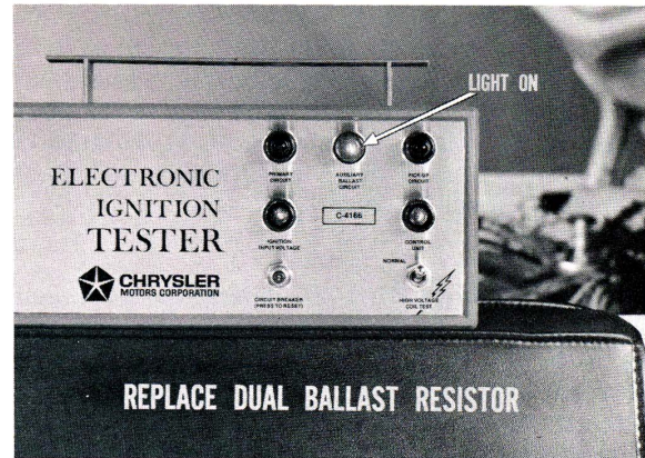
Fig. 21—This test only for five-ohm side
