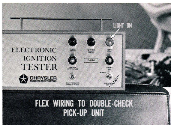
Fig. 23—Red light means pick-up must be replaced
