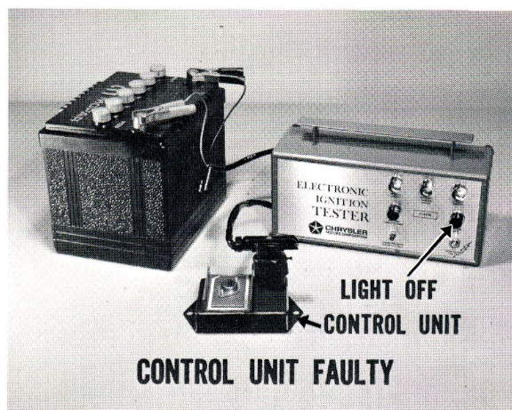
Fig. 27— If light is on, control unit is okay
