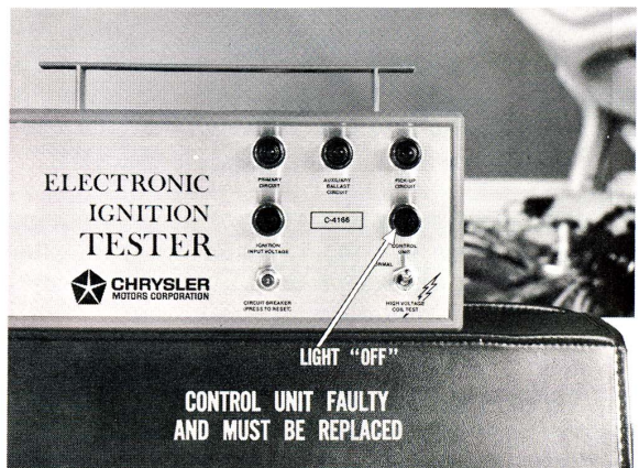
Fig. 19—Control unit test independent of others
